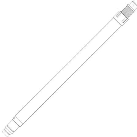
**1-3.4 Long Shore Strut Extensions.** When combined with a 12" hinged base plate and/or optional rigid or swivel base and ground plates, the 2', 4' and 6' strut extensions, figure 1-3, are
