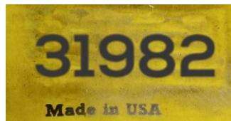
B. Starting in 1986 Paratech switched to a six digit serial number utilizing the first two digits of the serial number to indicate the year of manufacture. An air lifting bag with a serial number of 050644 was manufactured in 2005.
