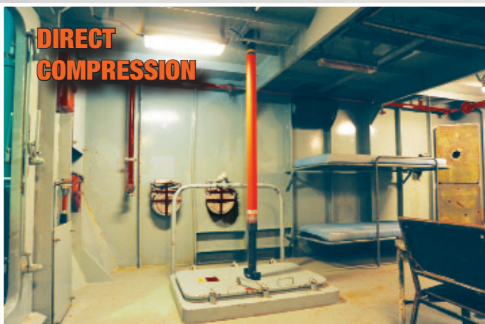
I-Type, can be used vertically or horizontally and is the simplest and strongest as it is parallel to the load axis (see table).
