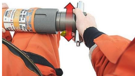
Figure: 4-2 Locking a Latch Connector to a Shore
