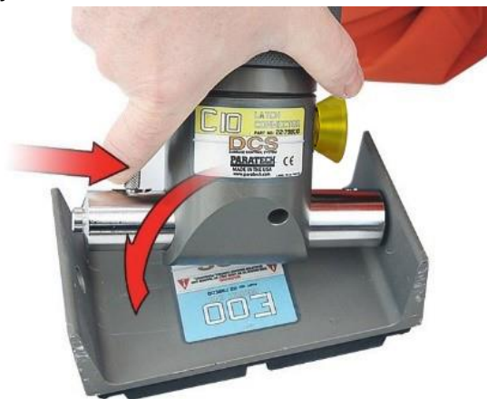
Figure 4-3: Attaching a Latch Connector to an End
