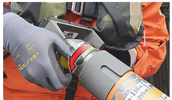
Figure 4-7: Locking the Shore in closed position
