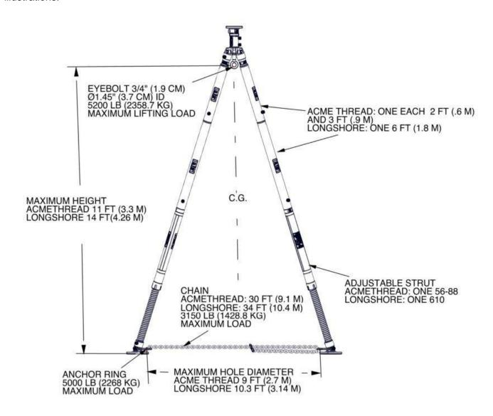
\* Dimensions represent the largest permitted component configuration for lifting.
