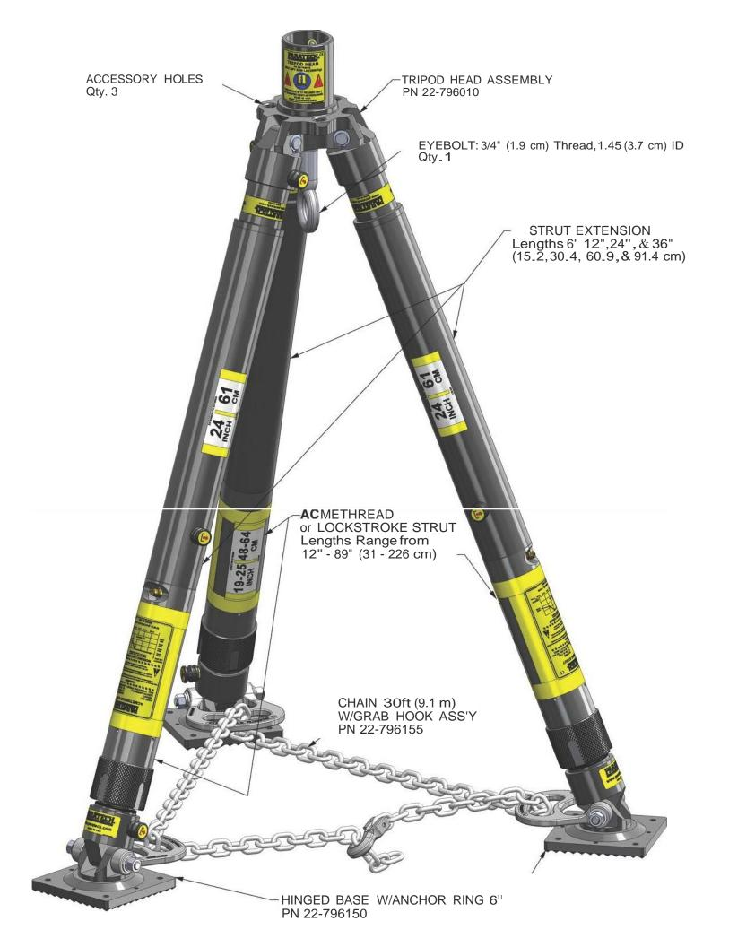
When setting up the tripod, always be sure to move the legs and bases from a maximum spread to a minimum of 2" (5.1 cm) toward the center of the triangle formed by the bases. Then attach the chain securely, causing it to be under tension. This will prevent the legs and bases from spreading while the tripod is under load.
