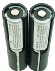
Figure 3: Four CR123A lithium batteries inserted into two adapter tubes.
