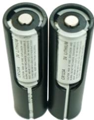
*Figure 2: Four CR123A lithium batteries inserted into two adapter tubes.*
